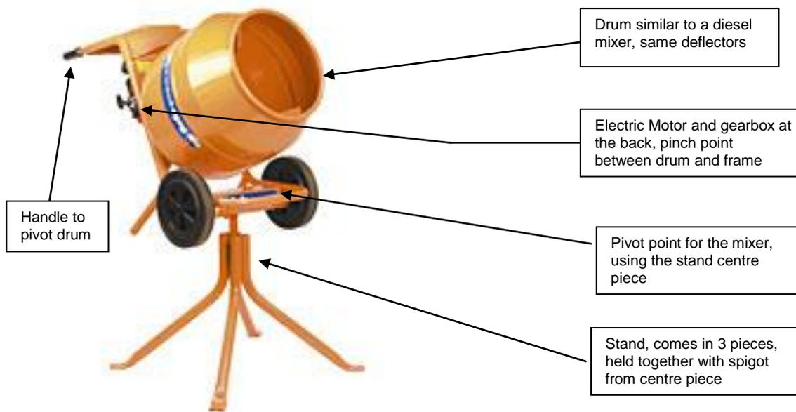
This photo shows an Electric Mixer, as assembled. The drum and motor have to be lifted onto the stand. This is a manual handling issue – needs a 2 –person lift.
