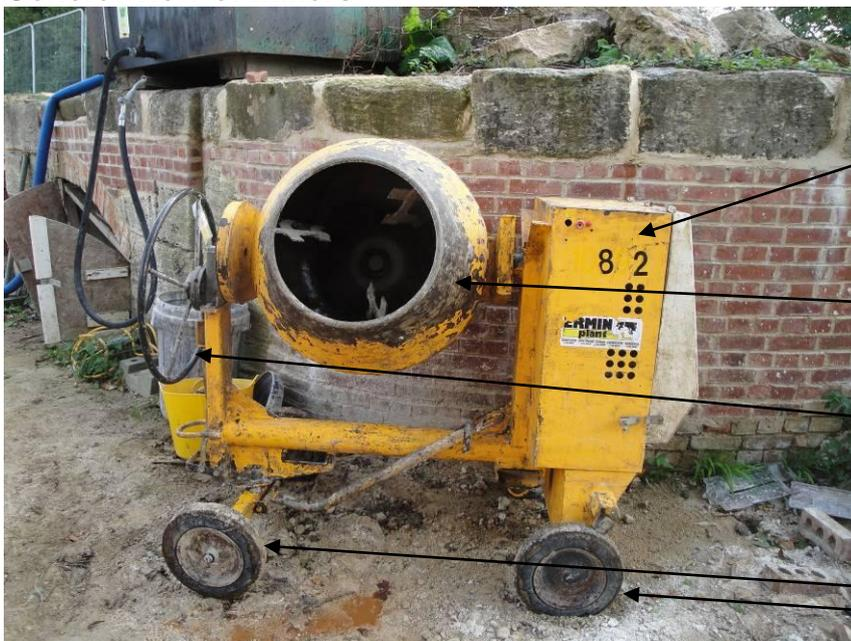
Diesel engine and gearbox under this cover
